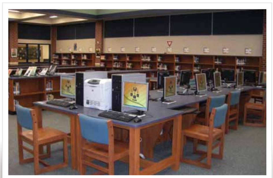
NComputing access devices are solid-state and contain no moving parts such as fans. This ensure a quiet work area for students and librarians.
